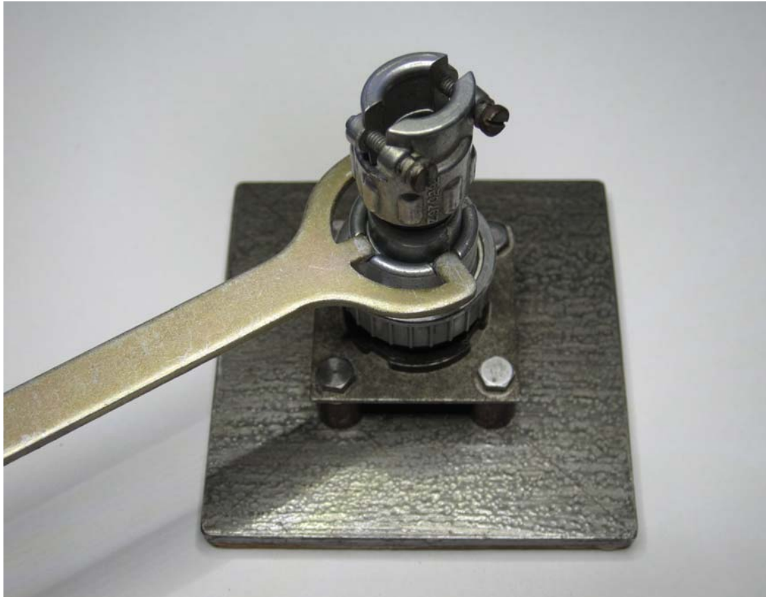
03) A Weald Electronics double-ended spanner undoing the outlet nut of a free connector held in the home brew jig.
